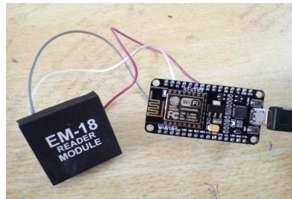
Fig 4 Connection Between RFID and ESP wifi Controller:
